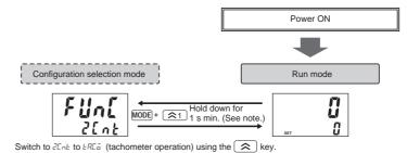
Note: The MODE key must be pressed before the <a>1</a> key.
