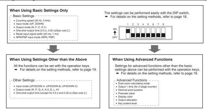
Note: 1. At the time of delivery, the H7CX is set to the 1-stage counter (2-stage counter for H7CX-AW\(\sigma\)/-A4W\(\sigma\) models) configuration.
