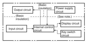
**Note**: All models except for H7CX-□D (models with 12 to 24-VDC power supplies) have basic insulation.
