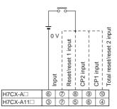
Operates when the contact turns  $\ensuremath{\mathsf{ON}}.$
