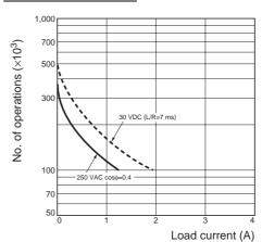
Reference: A current of 0.15 A max. can be switched at 125 VDC ( $\cos\phi$ =1) and current of 0.1 A max. can be switched if L/R=7 ms. In both cases, a life of 100,000 operations can be expected. The minimum applicable load is 10 mA at 5 VDC (failure level: P).
