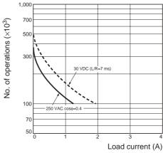
Reference: A current of 0.15 A max. can be switched at 125 VDC ( $\cos\phi=1$ ) and current of 0.1 A max. can be switched if L/R=7 ms. In both cases, a life of 100,000 operations can be expected. The minimum applicable load is 10 mA at 5 VDC (failure level: P).
