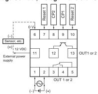
Note: Each output can be flexibly allocated to either stage 1 or 2 by setting in function selection mode.
