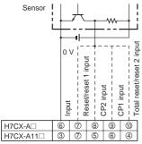
Operates when the transistor turns OFF.
