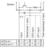
Operates when the transistor turns ON.
